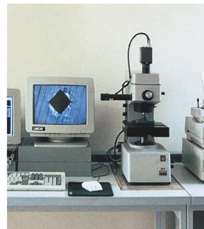
Figure 9: Automatic hardness tester (Protocolling of hardness values and hardness curve)
